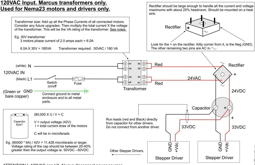
ATTENTION! 120VAC can kill. Always disconnect power sources when working on any electrical circuit. Use extreme caution when making connections. If you do not have the knowledge or understanding of electricity seek the advice of a qualified person. Capacitors can hold large amounts of electricity even when the power has been disconnected.
